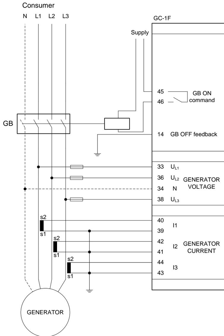
The AC current grounding can be made as required to s1 or s2.
