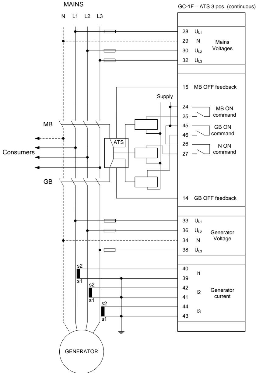
The GC-1F can operate ATS switches in Gen - Mains and Source - Source applications.
