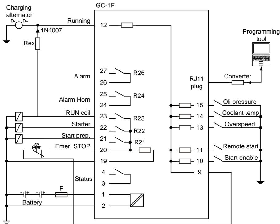
Term. 12 can be used as alarm input if not used for charger generator terminal D+
