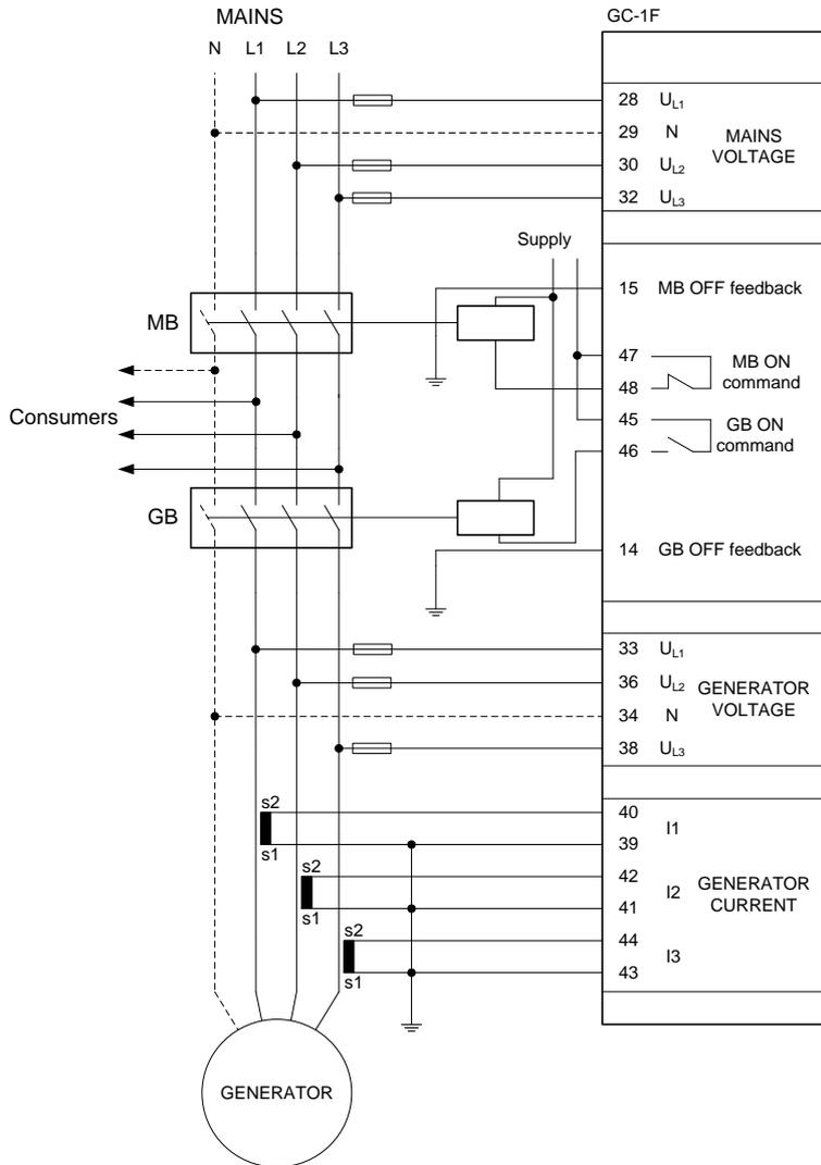
The AC current grounding can be made as required to s1 or s2.
